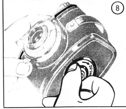
Turn the locking lever at the bottom to the right till both dots lie side by side (at "LOCK"). This pulls home and locks the top part.
