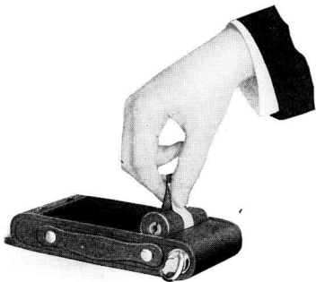
Fig. 2 Lifting out roll of exposed film.
