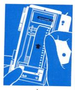
Draw out enough film for the narrow tongue to reach the winding spool easily. Then turn the spool by its milled ring until the broad slit and small film perforation lug are uppermost. Insert the film in the slit so that the lug engages in the second film perforation.
