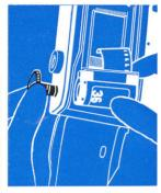
Draw out the rewind knob with the left hand as far as it will go and insert the film cassette. Push back the rewind knob.
