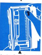
Now turn the winding spool in the direction shown by the arrow until about 1/ard. inch full width of film projects from the cassette.
