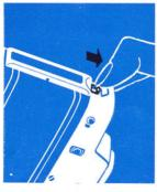
Open the camera back by sliding catch in direction of arrow.
