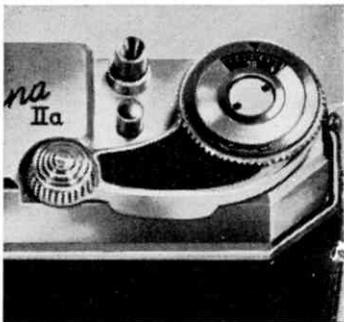
**3.** Draw out the film REWIND KNOB as far as it will go. Insert the film magazine in the recess under the rewind knob. The end of the magazine containing the crosspiece goes toward the rewind knob. Push in the rewind knob and turn it to engage the slot with the crosspiece in the magazine.
