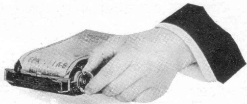
FIG. IV. Binding the Red Paper on Reel.
