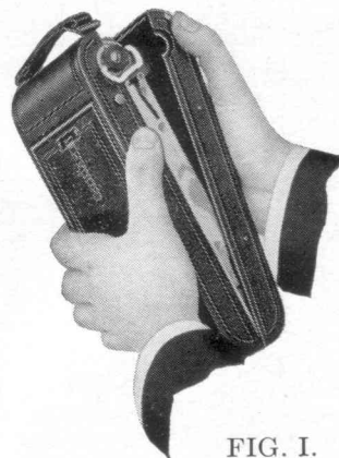
FIG. I. Removing the Back.
