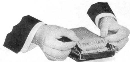
FIG. III. Threading Red Paper into Reel.
