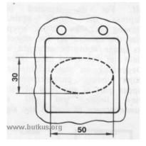
With the use of camera KIEV 88 TTL you can determine the exposure time and the diaphragm aperture with the aid of an exposure meter built into the prismatic view finder. Advantage and convenience of the TTL measurement system lies in the automatic control of all factors affecting the value of the exposure time. The field of measurement of the exposure time meter is in the central part of the view finder field of vision and has an oval shape ( ref. to the Figure). The exposure time meter ensures
