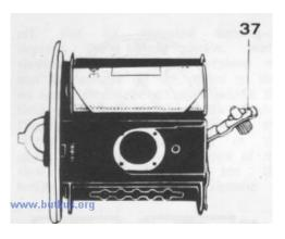
Remove transport mechanism 33 from the magazine. Turn plate 37, remove the spool with exposed film and glue the leader with a paper label.
