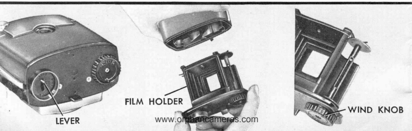
**3** Place the end of the full film spool between the fork of the **SPRING** pointed out by the word **LOAD** on the film holder. Push up against the spring; then swing the other end of the spool in and let it snap into the **HOLE**.
