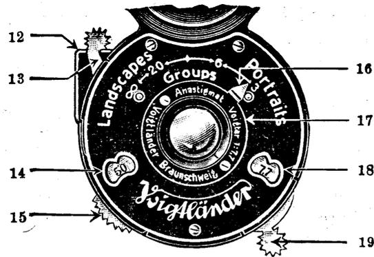
Fig. 5 Shutter with "Three Point" focussing
