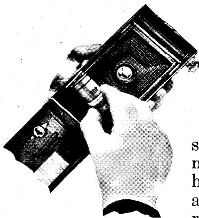
Lift up the spool holder nearest the hinged back and place the roll of film in it, springing out the flanges until the pins engage the holes in the spool. Make sure that the word "TOP" on the paper is on the side opposite the winding key.
