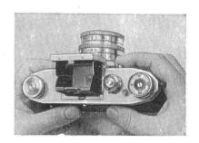
the picture, the knob should not be let loose until the shutter has run down. When set at "B", the shutter must be pressed as long as the exposure is to last. For the use of a wire release, the knob is provided with a thread into which the release can be screwed. A special wire release is supplied with the camera for long time exposures in the T-setting (e. g. in night photography).
